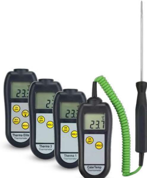
**INSTRUMENT OPERATION** - Where applicable, connect a probe via the socket located at the top of the instrument. Switch the instrument on and apply the tip of the probe to the substance or medium to be measured. The instrument reading may take a few seconds to stabilise, depending on the nature of the measurement and sensitivity of the probe.
